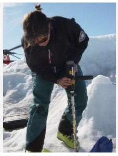
Leigh drills a hole in order to install a pole on the glacier's surface. Image courtesy of Leigh Stearns.
