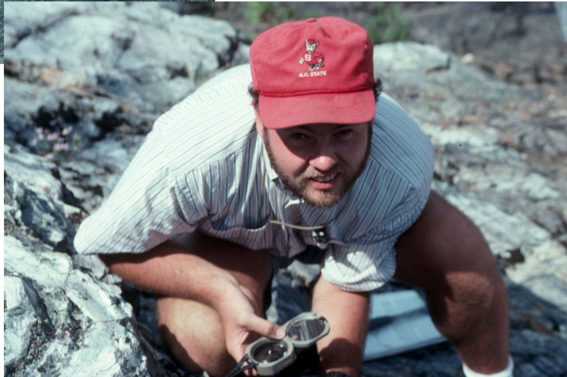
Measuring strike and dip with a Brunton compass
