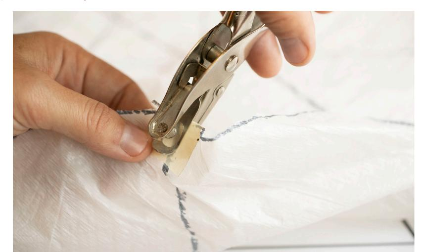
Here's the hole through the masking tape. Repeat this for each of the corners.
