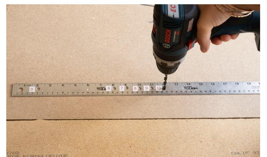
Here is a close up of hole location. The numbers represent the radius of the circular canopy.
