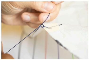
The intersection of the straight line with the edge of the canopy has shroud lines tied to it.
