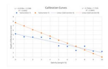
You measure a depth of the marking line of 3.9 cm for Salinometer A, and 5.0 cm for Salinometer B. To the nearest tenth of a percent, estimate the salinity of the sample. You will receive credit for being within 0.5%.
